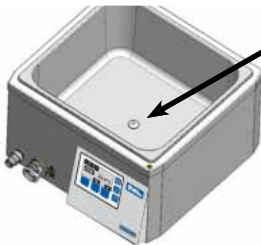
Figure 3-2— Thermal Beads Reservoir Plug
